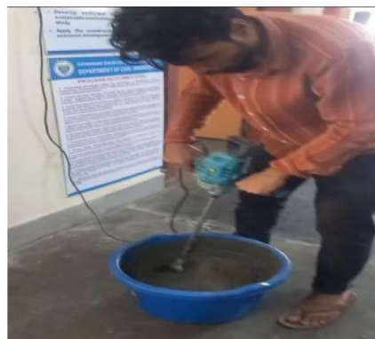
Mixing foam and cement mix
